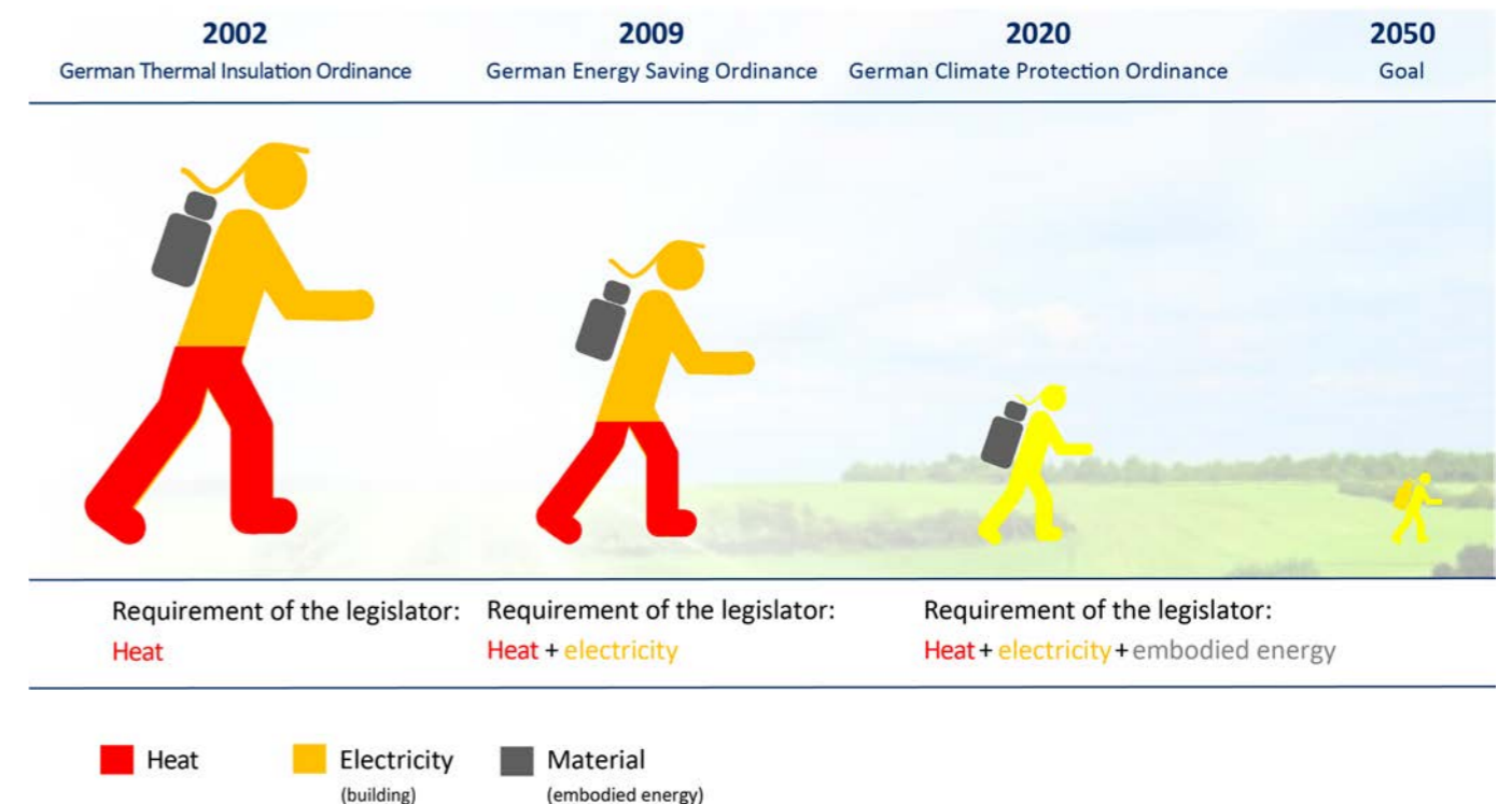
Fig. 7 – From the German Thermal Insulation Ordinance to the German Climate Protection Ordinance – CO 2 emissions in non-residential buildings (offices) balanced over 50 years of operation; Source: Drees & Sommer, Dr. Peter Mösle
